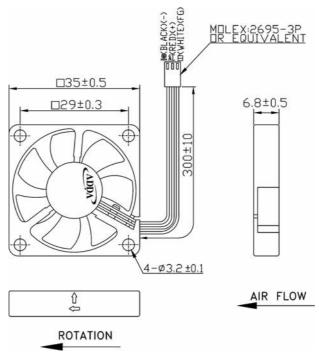
LEAD WIRES: UL 1571, AWG28, L = 300 +/- 10 mm Red = positive; Black = negative.
